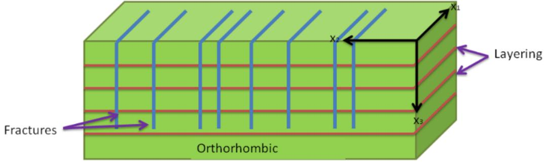
Fig. 1. Orthorhombic symmetry formed by 1 group of fractures embedded in VTI background.
