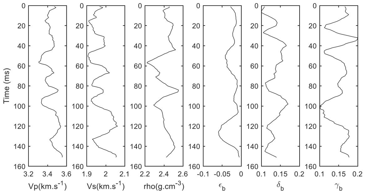
Fig. 3. A well log model referred to VTI background parameter curves. P- and S- wave velocity  $V_p, V_s$ , density  $\rho$ , Thomsen parameters  $\epsilon, \delta, \gamma$ .
