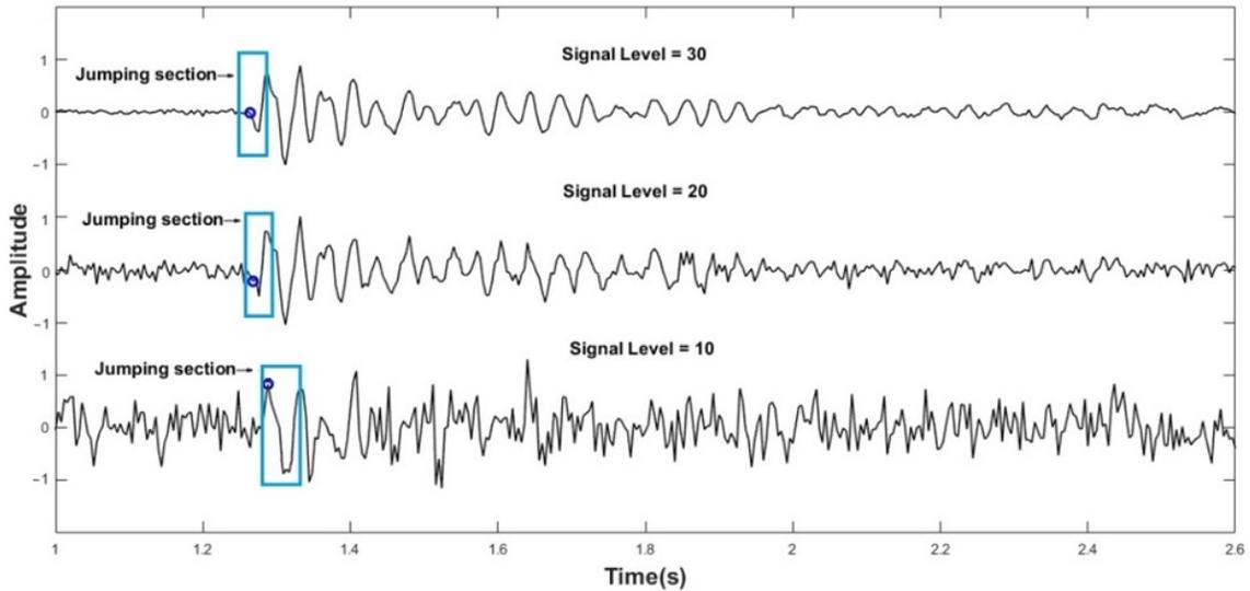
Fig. 7. The results of the first break picking method on synthesized traces with signal levels = 30, 20, and 10.
