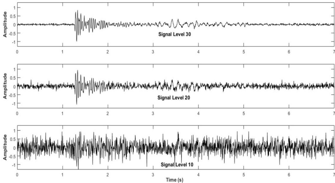
Fig. 6. The synthesized traces with signal levels = 30, 20, and 10.
