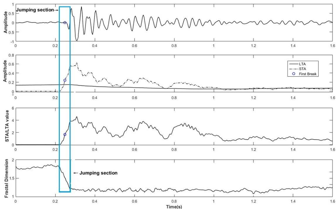
Fig. 5. The first break picking, the STA and LTA, the STA/LTA ratio, and calculated fractal dimension for a seismic trace.
