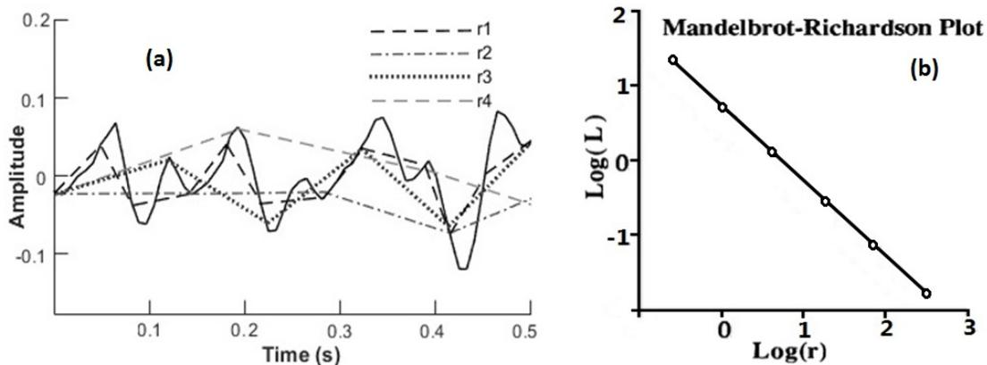
Fig. 2. a) The sketch displays how to calculate the length of a signal using step sizes ( $r_i$ ) based on the divider method. b) A Mandelbrot-Richardson plot, which is obtained by plotting the logarithm of the signal length versus the logarithm of the corresponding step size.
