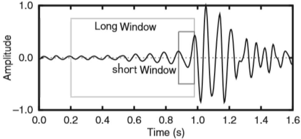
Fig. 1. Moving short and long time windows on seismic trace to calculate the STA and LTA.
