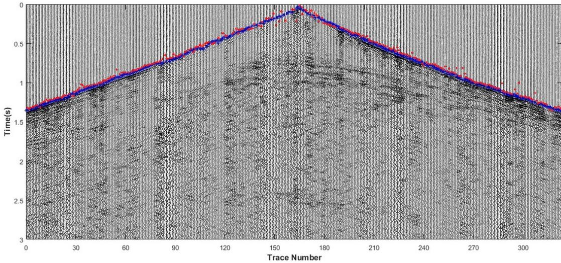
Fig. 8. The results of the first break picking on a shot gather (obtained from a seismic project in the west of Iran) by the STA/LTA fractal dimension algorithm (blue), and STA/LTA algorithm (red).
