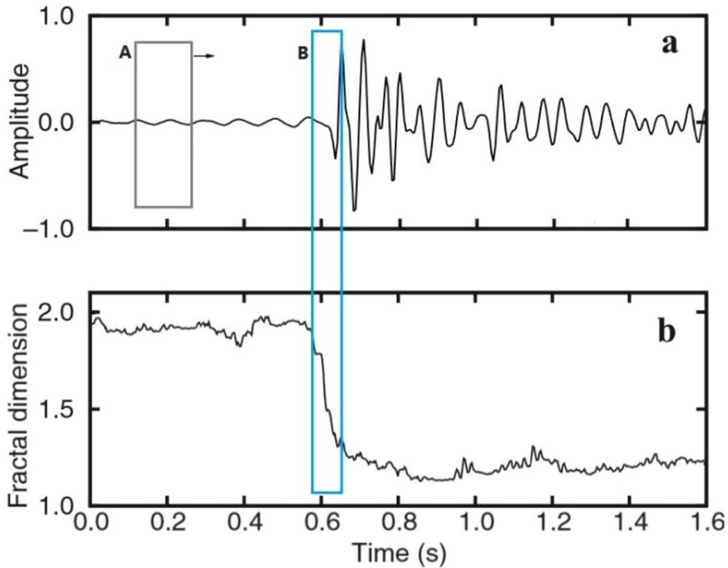
Fig. 3. a) A is a moving time window along the seismic trace which is used in the calculation of the fractal dimension. b) Fractal dimension of the seismic trace (in a). The blue window shows the jumping section in fractal dimension.
