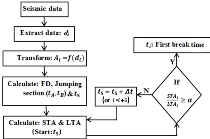
Fig. 4. The STA/LTA fractal dimension algorithm.
