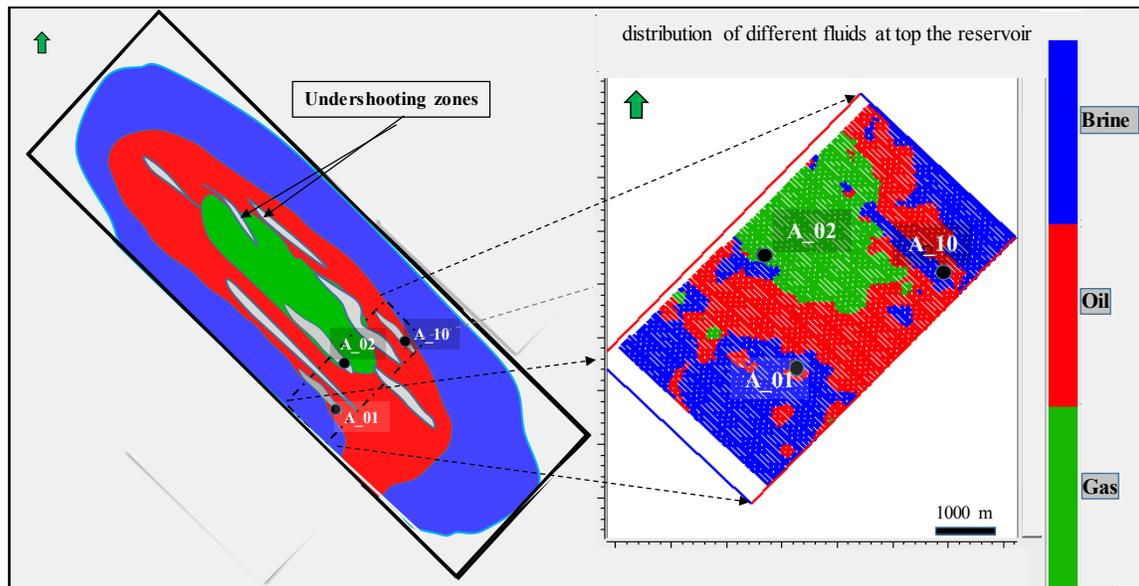
Fig. 9. Spatial discrimination map of different fluids at the top of the reservoir based on well data modeling is present on the left side to compare with the map resulting from the presented method (right side). The slight difference between the two maps is due to undershooting areas (gray polygons). In addition, the spatial resolution of the map resulting from seismic data between boreholes is more than the map created from sparse well data modeling.
