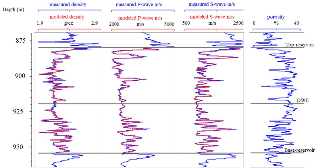
Fig. 3. Measured well log data (blue) and predicted data (red) along unconsolidated reservoir at A-01. Track 1 shows the measured and modeled density. P- and S-wave velocities are shown along tracks 2 and 3, respectively. The total porosity log is present along track 4.
