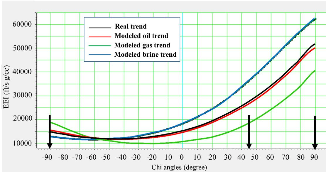
Fig. 6. EEI values changes from  $-90^\circ$  to  $+90^\circ$  of Chi angle for the different scenario of fluid type at the top of the reservoir calculated by the well A-01 data. Since the well A-01 has been drilled in the oil, the trends of EEI for the oil scenario and the real one are almost similar. Black arrows indicate angles  $-90^\circ$ ,  $+45^\circ$  and  $+90^\circ$ .
