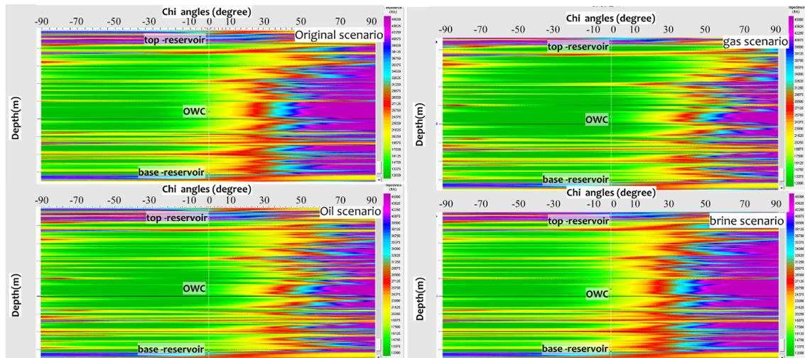
Fig. 5. EEI spectrum for different scenarios (original, 100% oil, 100% gas and 100% brine) using eq. (2). The color scale indicates EEI values at different depth and chi angles. The different EEI spectrum for different scenarios is clear.
