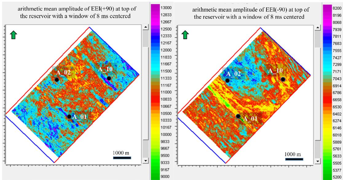
Fig. 7. EEI changes amplitude map for two Chi angles selected according to fluid EEI template of different saturation scenarios. The EEI template is created based on rock-physics modeling and FRM.
