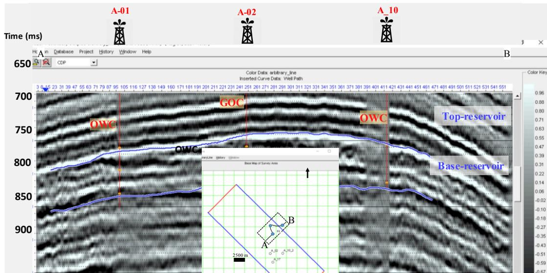
Fig. 2. An arbitrary seismic section of the field. The reservoir is located between two blue horizons. The base map shows the full coverage of seismic data. The blue points represent well locations. The dotted square indicates seismic data available for this study, and the black line shows the arbitrary line path on the map.
